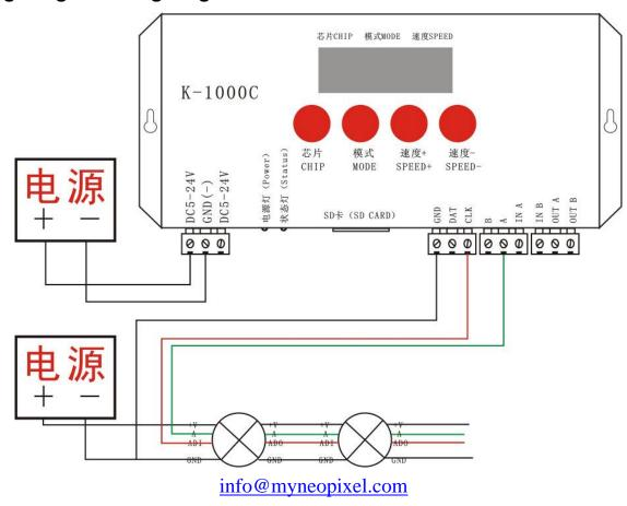
1. Like the above diagram, wired the line and start the controller, press "CHIP" and "MODE" at the same time switch to coding mode, adjust to Chip: 61 that is UCS512A or B coding mode, as below:
